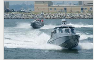
FORT MONROE, Va. (July 20, 2011) Autonomous Maritime Navigation 1 (AMN1) and Autonomous Maritime Navigation 2 (AMN2) patrol for intruders during Trident Warrior 2011. The experimental boat can operate autonomously or by remote. The Trident Warrior experiment, directed by U.S. Fleet Forces Command, temporarily deploys advanced capabilities on ships to collect real-world data and feedback during an underway experimentation period. U.S. Navy photo by Mass Communication Specialist Seaman Scott Youngblood.
