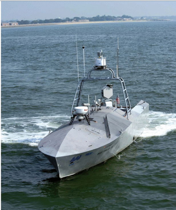
A common unmanned surface vehicle patrols for intruders during Trident Warrior 2011 July 20 at Fort Monroe, Va. The experimental boat can operate autonomously or by remote control.
